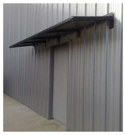
Galvanised and painted steel framework. Polycarbonate Glazing. Easily fixed to wall – no uprights. Integral rainwater drip flashing. Dimensions: 1.0m deep x any length. Can be manufactured to any size. **2.0m long Canopy(3 person)**
